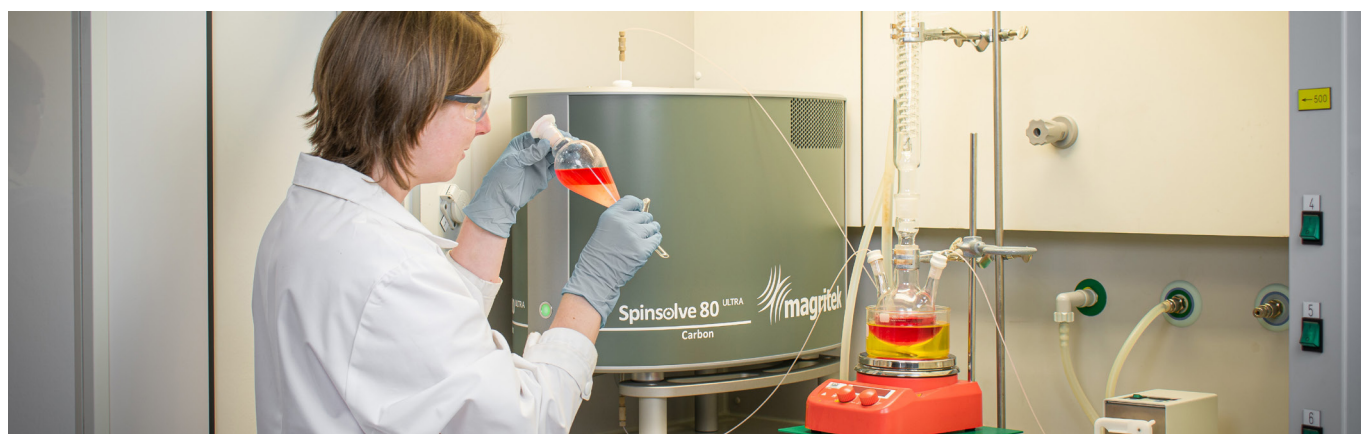
Figure 1. Spinsolve NMR spectrometer used in the chemistry lab for quick analyses of products. The typical presence of protonated solvents in the sample requires the use of solvent suppression and carbon decoupling methods to acquire the spectra of analytes of interest.
