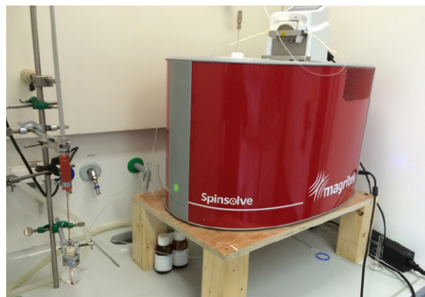
Figure 1. Spinsolve NMR spectrometer set in a fume hood to monitor the hydrolysis of acetic anhydride.
