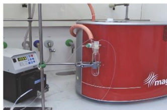
Figure 1. Experimental set up. (a) NMR magnet; (b) NMR flow cell; (c) Peristaltic pump to provide the continuous flow of the reaction mixture through the magnet bore. The NMR spectrometer is outside the fume hood and cannot be seen in the pictures.
