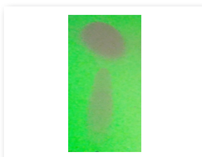
Figure 4: Silica TLC plate of the mixture run with dichloromethane and visualized with UV light.
